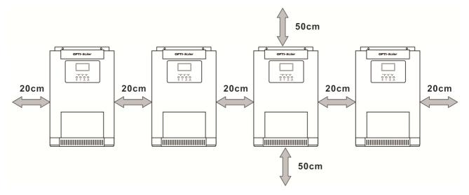
**NOTE:** For proper air circulation to dissipate heat, allow a clearance of approx. 20 cm to the side and approx. 50 cm above and below the unit. Be sure to install each unit in the same level.
