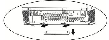
Step 5: Install new parallel board with 2 screws tightly.
