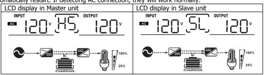
Step 5: If there is no more fault alarm, the parallel system is completely installed. Step 6: Please switch on all breakers of Line wires in load side. This system will start to provide power to the load.
