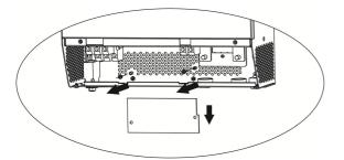
**Step 4:** Remove two screws as below chart to take out cover of parallel communication.
