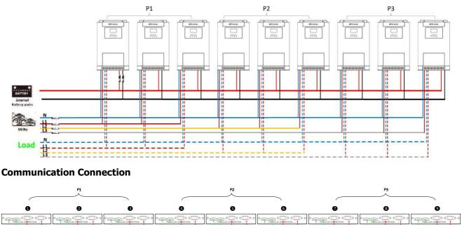
Three inverters in one phase, three inverters in second phase and two inverter for the third phase: **Power Connection**
