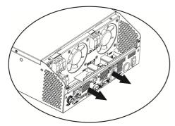
**Step 3:** Remove two screws as below chart and remove 2-pin and 14-pin cables. Take out the board under the communication board.
